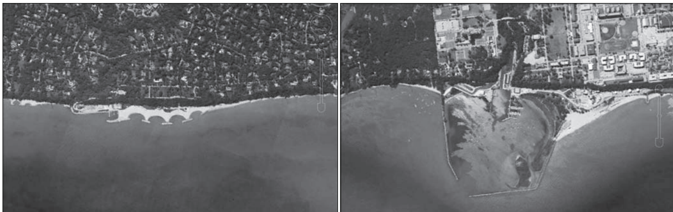
Figure 7. View of the largest headland-protected beach in Lake Michigan at Forest Park Beach in Lake Forest, Illinois (above). The system lies within the surf zone, extending about 400 ft from the bluff toe into the lake. In comparison, 3.5 miles updrift (north) is Great Lakes Naval Training Center Harbor (below) that was, for nearly a half century, a total littoral barrier. The breakwaters, built in 1923, protrude 2,400 ft into Lake Michigan. Between 1923 and 1976, approximately 2.5 million cu yds of sand was impounded in the harbor and on its updrift side (Chrzastowski and Trask 1995). 2007 Google photos both to same scale.
